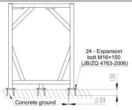
Fix the base frame at the desired position with four M16×150 expansion bolts and the pre-tightening force of the bolts should be 125 Nm.
