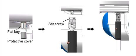
1. Remove the protective cover and loosen the set screws at the shaft side of the universal
